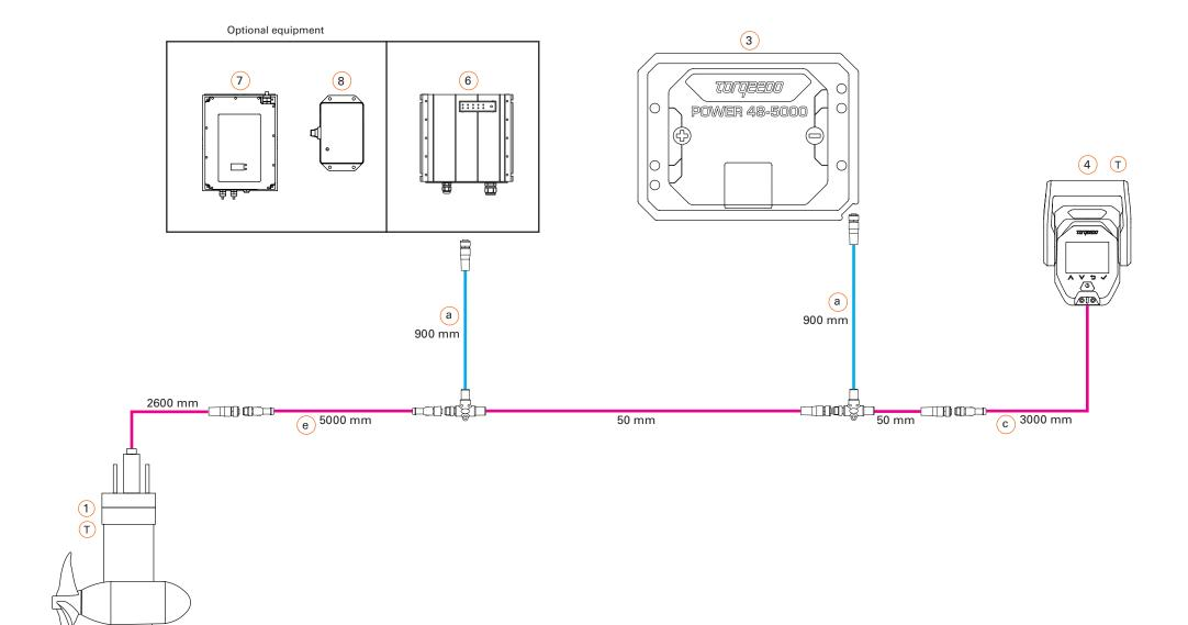
Backbone TorqLink, 8 pin data cable
