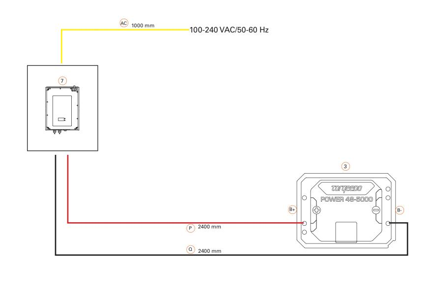
Installation Drawing: 108 Version 1.0 Power cable connection
