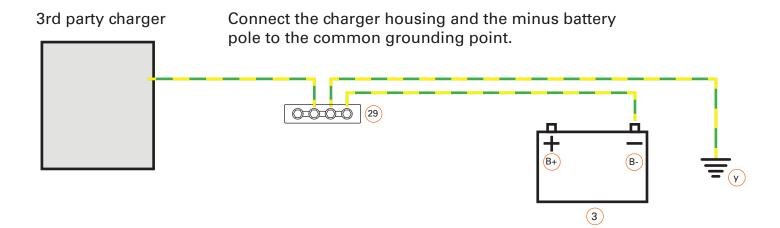
Installation Drawing: 140 Item number: 039-00511, Version 1.0 Data cable connection
