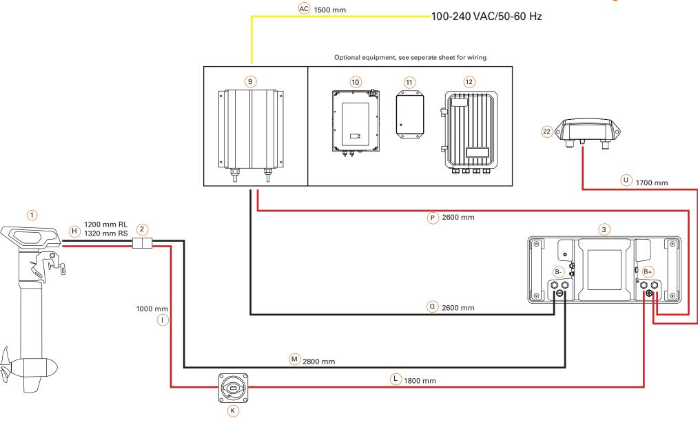
Positive power cable Negative power cable Positive charging cable Negative charging cable
