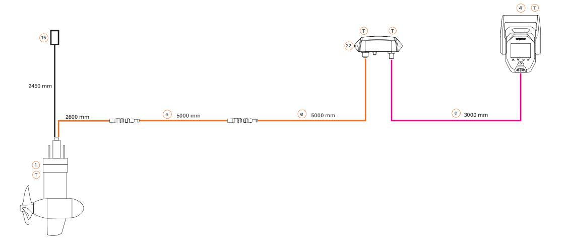
Backbone TorqLink, 8 pin data cable
