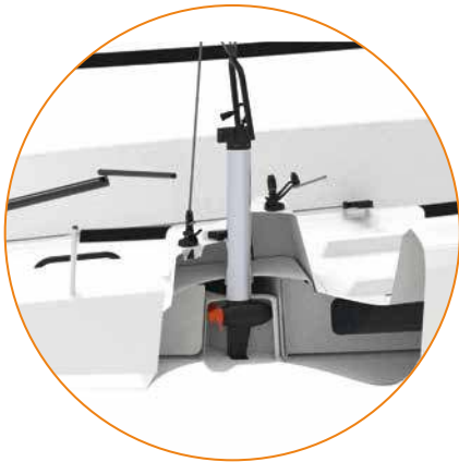
Up position: When it's time to sail, simply pull up the motor and secure the line. The hull is completely flush and ready for racing while the motor and battery are securely stowed. The lightweight lithium-ion battery is easy to remove when it's time to charge.
