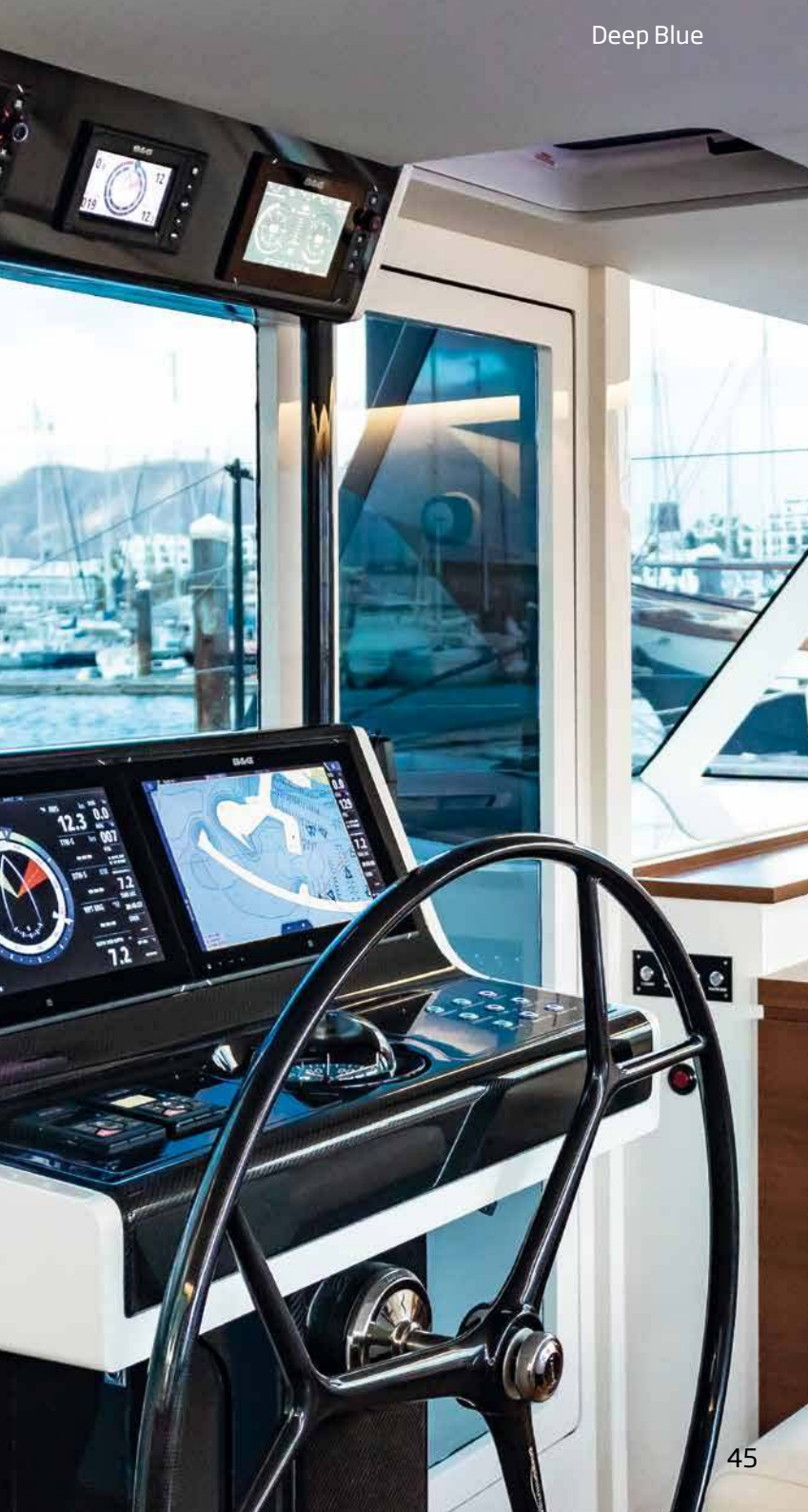
Drive screen: All important information needed while motoring. You can choose to display or hide the information line at the top.
