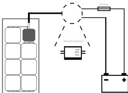
ALLinONE modules are supplied with a flexible cable resistant to weathering that can be directly connected to the positive and negative poles of your battery. Alternatively, the cables may be attached to the positive and negative bus bars or posts, to avoid wiring clutter at the batteries. The electronics are configured at the factory, the right model must be ordered for the chosen battery type.
